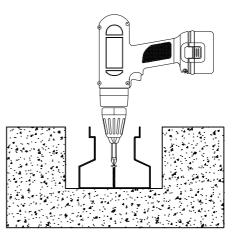
4. Make Sure the surface of the housing is flushed with the ground
